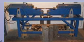
Full-scale CT rotating-bending fatigue testing machine, shown with 1.25" diameter sample.
